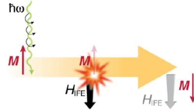
**Figure 1.** The magnetization ( $\vec{M}$ ) switching by a short and intense circularly polarized laser pulse. Shortly after the pulse, magnetization collapses due to heating. During the cooling,  $\vec{M}$  restores along the effective field.
