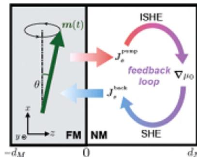
**Figure 3.** The interconnection between the magnetization precession and the electric current  $\bar{I}_c = \nabla \mu_0$  ( $\mu_0$  is an electrochemical potential) via spin pumping, the ISHE, the SHE and spin backflow closed in the feedback loop.
